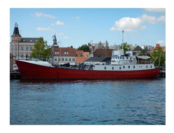
Christoffer has been operated within the Offshore Wind segment for many years and carried out surveys of various kinds such as: Site scan, Multibeam, ROV and Video, Bottom Sampling, Diving Platform, POD Handling, Bird observation platform, Trial Fishery and Guard Surveys.
